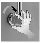
**3.** Be sure shower wall is clean where drill-free suction cup will mount. Firmly press diverter knob against the wall and turn suction cup knob clockwise until you hear a click.
