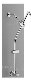
2. Apply fresh pipe tape in clockwise direction to existing pipe nipple, then mount new rail by screwing hex nut clockwise onto existing pipe nipple. Included washer should be inside hex nut before threading onto pipe nipple. Tighten hex nut with crescent wrench to ensure snug fit.
